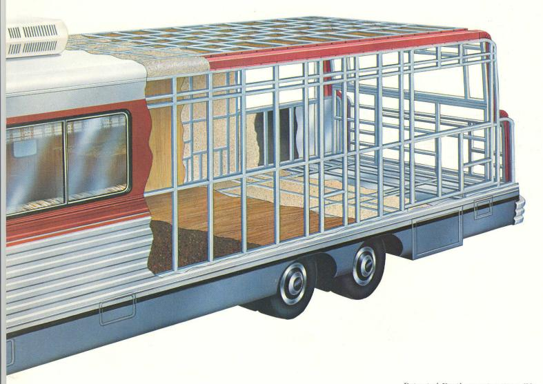
Patented Barth construction (No. 3,282,603) features interlocking, aircraft riveted, .062" aluminum extrusions and sidewall metal of .040" aluminum. Roof metal is one piece .032" aluminum. All models feature fully-insulated walls, ceilings, and floors.
