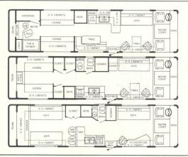
**34T.** 454 C.I.D. V-8 engine; 219" W.B.; 14,500 lb. GVWR chassis with tandem rear axle (5,200 lb. GAWR) and driver-controlled air lift suspension; Disc brakes on front and drive axle, drum and shoe on tandem axle; Tires: 8.00 x 19.5; Overall width 93"; Overall height 118"; Interior height 78"; Rear axle ratio 4.56.
